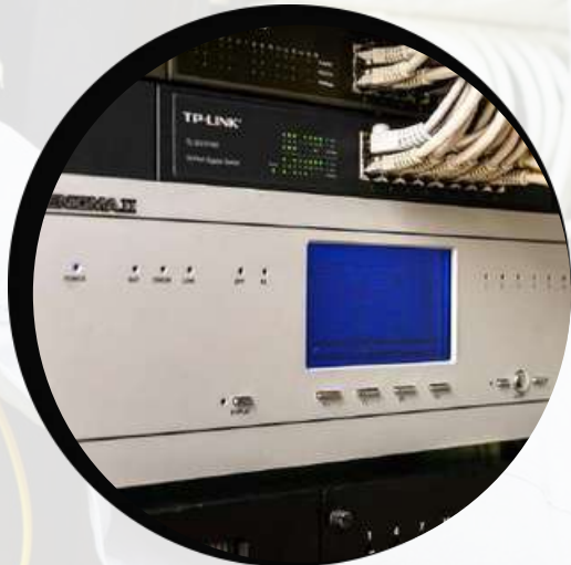
Military grade ENIGMA II signal receiver to secure incoming IP signals with embedded cards.
